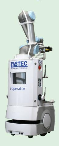
CASTEC i-Operator, an autonomous vehicle integrated with the collaborative 6-axis robot, and start with the application for semiconductor worldwide.
