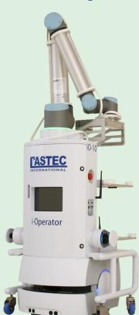
CASTEC i-Operator, an autonomous vehicle integrated with the collaborative 6-axis robot, and start with the application for semiconductor worldwide.
